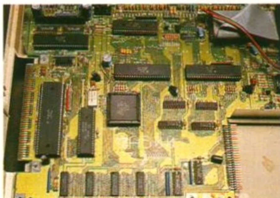
You should now have something resembling the above photograph in front of you. Don't be too alarmed if there are slight differences – there are four revisions of the A500; rev 3, 5, 6 and 7. All of them can be updated, but the difficulty and expense grows with the age of the machine – and as I can't get hold of a revision 3, I cannot guarantee that these methods work, so I'll be ignoring it this issue. The revision is printed on the board at the left-hand side, near the words 'B52 Rock Lobster'.
